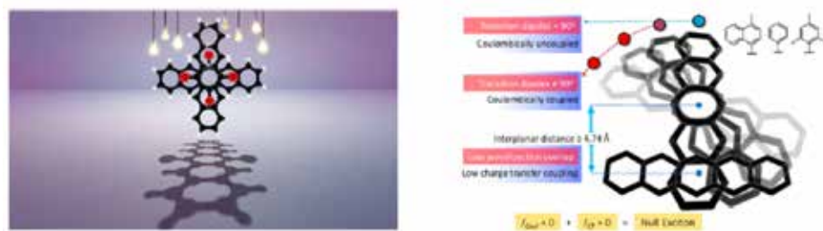
Figure 1. (a) Pictorial representation of Greek-Cross (+) orientation resulting in monomer-like optical properties. (b) Pentacene dimers depicting correlation of Coulombic (J) coupling with rotational angle and aryl groups substituted in the 6,13 positions of pentacene for attaining the orthogonally cross-stacked architecture.
